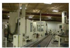
machining cell consisted of two Berthiez VTL's and a Forrest Line machining center utilizing 9 pallets and a motorized set-up station. Between the two VTL's was a CNC-programmed rail-guided vehicle that shuttled the pallets within the cell.
